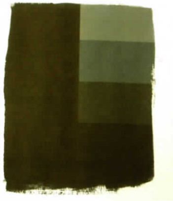
Figure 6-9 Develop normally. Develop the print normally; find the time for maximum black.
