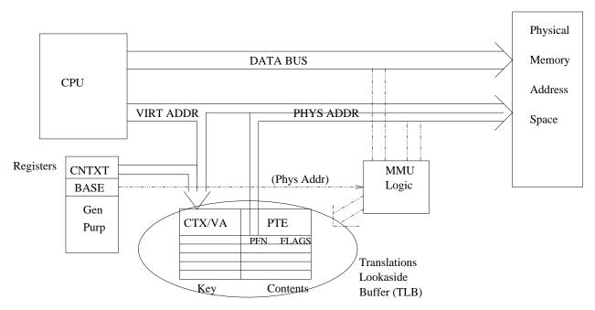
Aside: The X86 is a CISC (Complex Instruction Set) architecture in which the hardware handles all aspects of ATC/TLB operations, including "walking" the page tables to load a PTE, and the eviction strategy for old TLB entries. On some RISC (Reduced Instruction Set) architectures, TLB/ATC management is handled by the kernel. A TLB miss causes a fault to be raised, and the kernel must determine the PTE and manually load it into the ATC/TLB.
