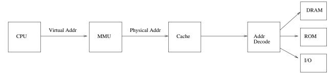
Since the operating system kernel has sole access to the MMU's lookup tables, it has the ability to completely control the view of memory a given process can see.
