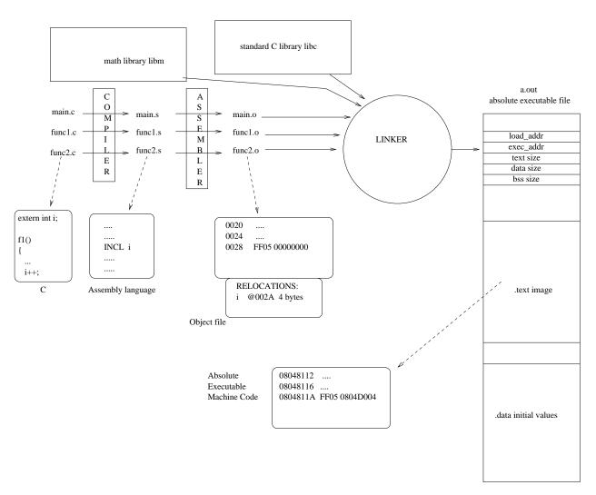
The compiler proper takes C code, passing it through the macro pre-processor, and compiles it into symbolic assembly language. By using the -S option to cc, we can halt the process before the assembler and linker are invoked, and view the intermediate assembly language file, which will have a .s extension.
