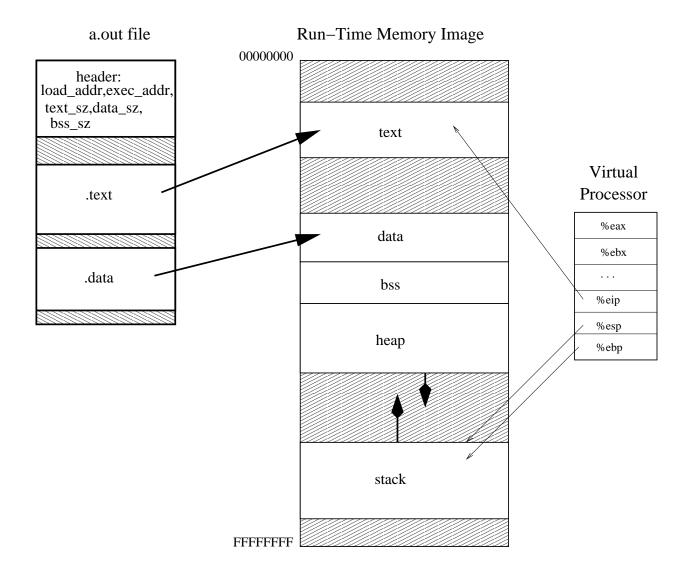
The **bss** section contains all un-initialized global variables. The C language specification states that all such variables, lacking an explicit initializer, must be initialized by the operating system or C run-time environment to 0.
